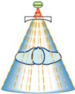
Non-contributing X-rays Absorbed with IntelliBeam Filter
