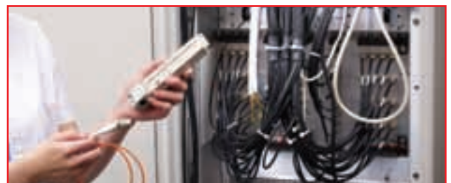
Figure 2. Ingenia's DirectDigital miniaturized electronics that are fitted in the coil (in the technician's hand) replace the large electronics rack.
